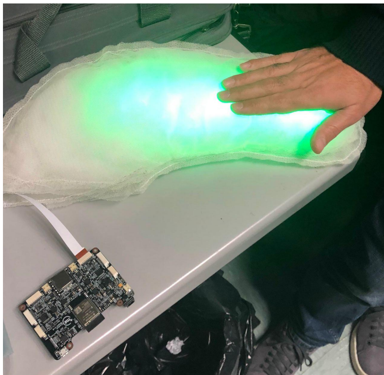
Figure 20. Preliminary test of the touch sensors; the device correctly detects the human touch and responds with a green light.
