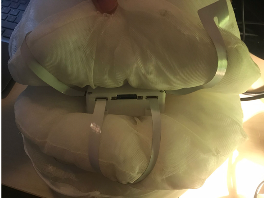
Figure 19. Main Board module inside the pillow. The picture shows also the SAMs connections.
