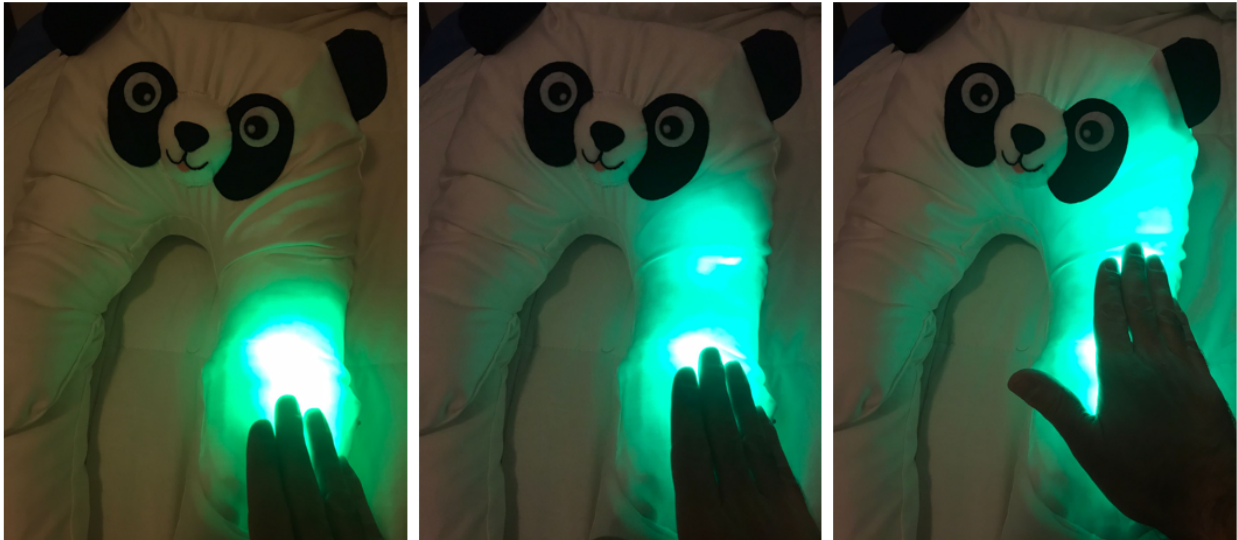
Figure 21. Test of the final, assembled device: the four paws correctly detects the human touch.
