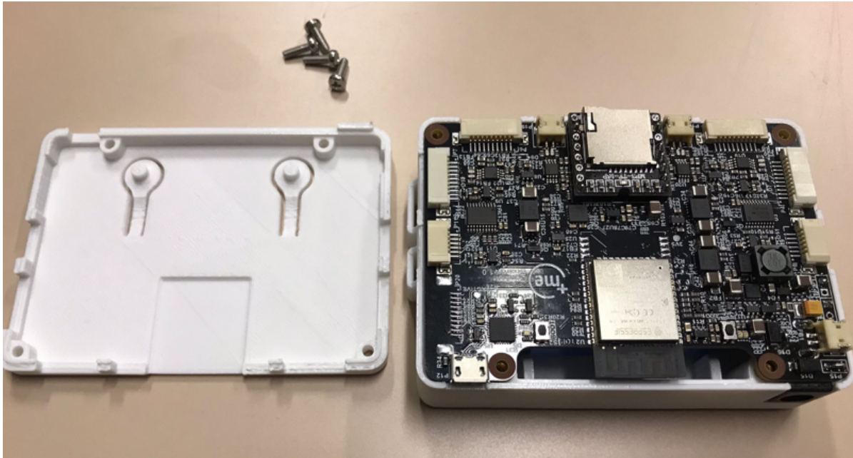
Figure 17. Main Board insertion in the box.
