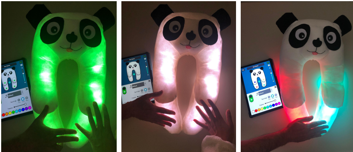
Figure 4. Top: the new control App, through an intuitive GUI, allows the user (a therapist or a caregiver) to customise several PlusMe features: for example he/she can select the colour of the light, its temporal pattern (steady or pulsating) and the sound to be emitted when PlusMe detects a touch. Bottom: examples of PlusMe different configurations.
